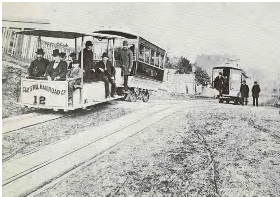
Figure 3. Hallidie's original cable streetcar on Clay Street in San Francisco in September 1873. Note the slot visible in the middle of the tracks where the grip from the cable car attached to the underground cable. 23
