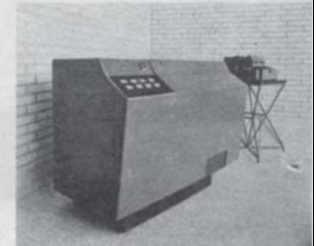
The RW-300 digital control computer has broad applications in automatic process control, data reduction and test facility operation
