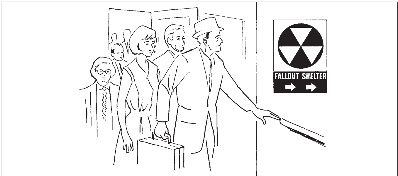
BASEMENT SHELTER , designed by the Office of Civil and Defense Mobilization, is recommended for protecting the average family from radioactive fallout. The 13 x 8-foot shelter can be built of concrete blocks for about $300 on a do-it-yourself basis, somewhat higher if contracted. (OCDM Photo)
