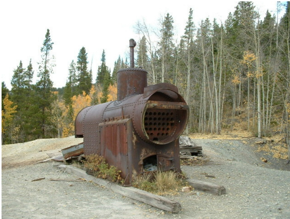
Figure E 5.2.23. A Pennsylvania boiler at the Ouray Shaft, Summit County, Colorado. Source: Author.
