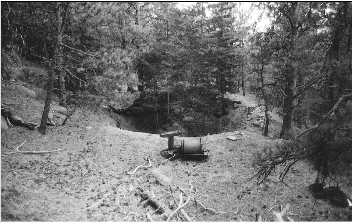
Figure F 3.1. An abandoned horse whim stands adjacent to a collapsed prospect shaft near Summerville. The whim is an important historic resource because few currently remain. Source: Author.
