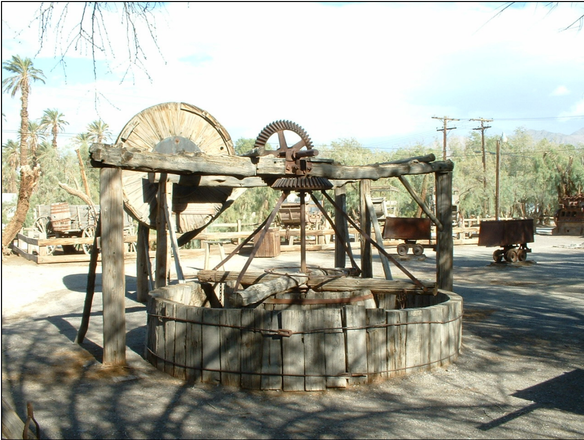
Figure F 6.16. When capital and resources permitted, mining outfits constructed arrastras that were powered by water. This unit at the Death Valley Museum illustrates the drivetrain, capstan, and sidewalls typical of power-driven arrastras. Source: Author.
