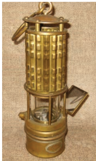
An improperly used Wolf key-lock safety lamp, similar to this lamp from the History Colorado collection, led to the explosion. H.4178.1
