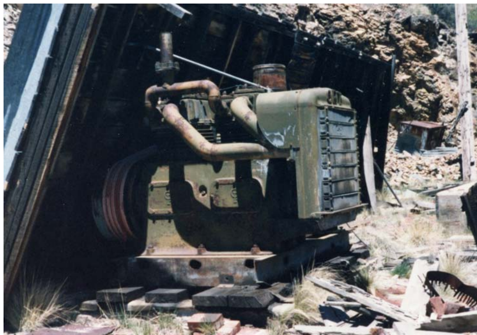
Fig. E.II.45 A three-cylinder V-cylinder compressor, belted to an electric motor, Gold King Mine, Cripple Creek. By the 1930s, capitalized mining companies in Colorado began to employ V-cylinder compressors, such as in this photograph. The compressor design was based on large-displacement truck engines and featured a radiator for cooling. Eric Twitty, taken 1998.
