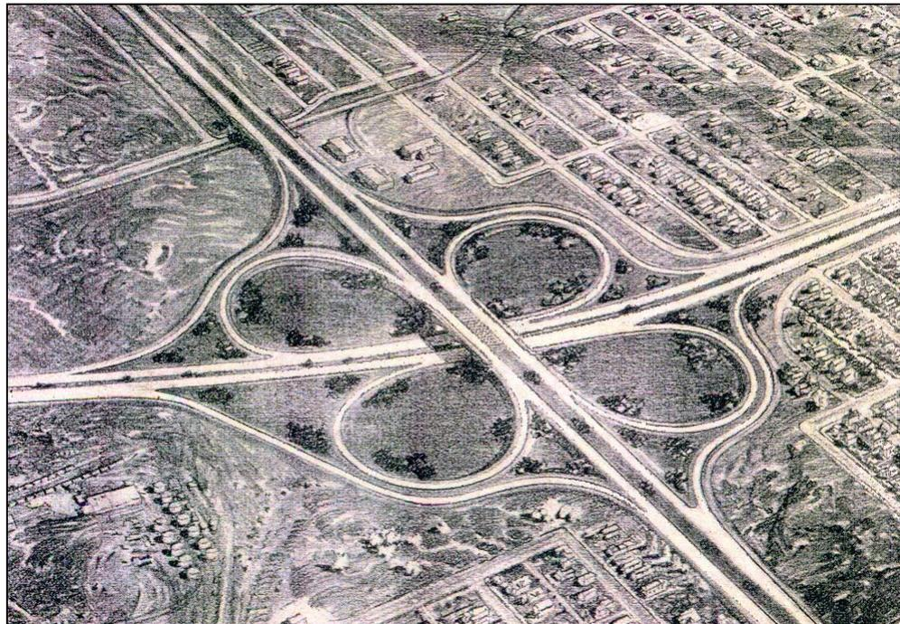
**Figure 51.** By the 1940s, the freeway cloverleaf interchange came to symbolize the future of Colorado highway development. Shown here is an artist's rendering of the proposed 46<sup>th</sup> Avenue interchange in the 1944 plan for Denver's Valley Highway. Source: Hermesen Consultants, Vol. I, 2000:12.
