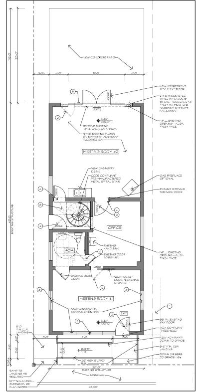
Figure 1. This 2018 construction drawing prepared for the remodeling and reuse of the building shows the interior floorplan. East Main Street is at the bottom of the drawing. The partial basement is only under the center part of the building. SOURCE: Sarah Weddington Architectural Services, The Ranger Station Renovation, construction drawing, January 12, 2018.
