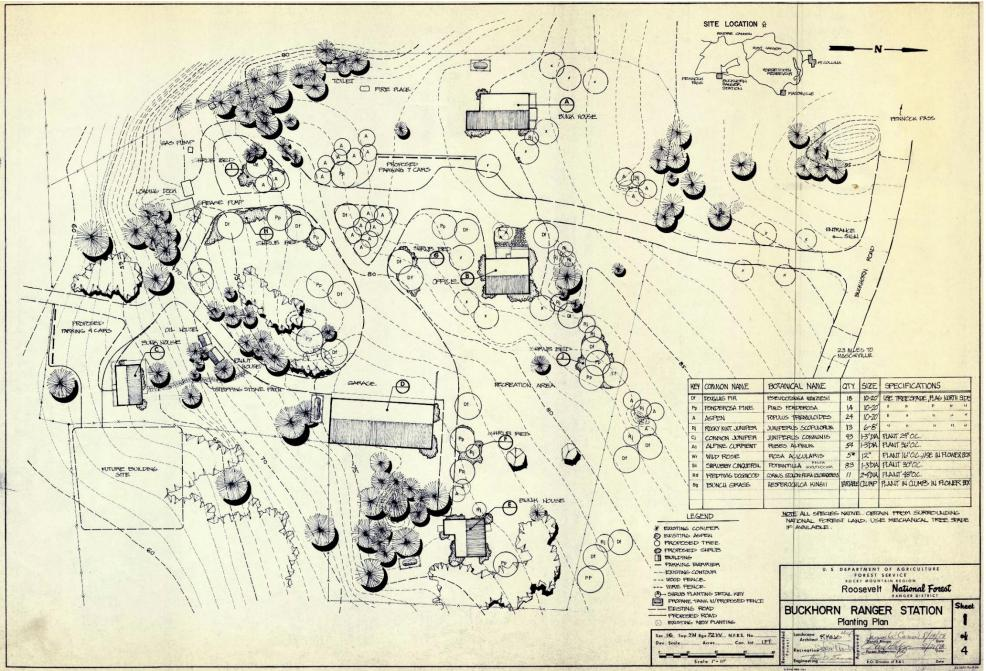
Figure 7m. United States Forest Service (1978) Development Plan of the existing site and plans for additional plantings, ground features and parking areas. These plans did not come into fruition.
