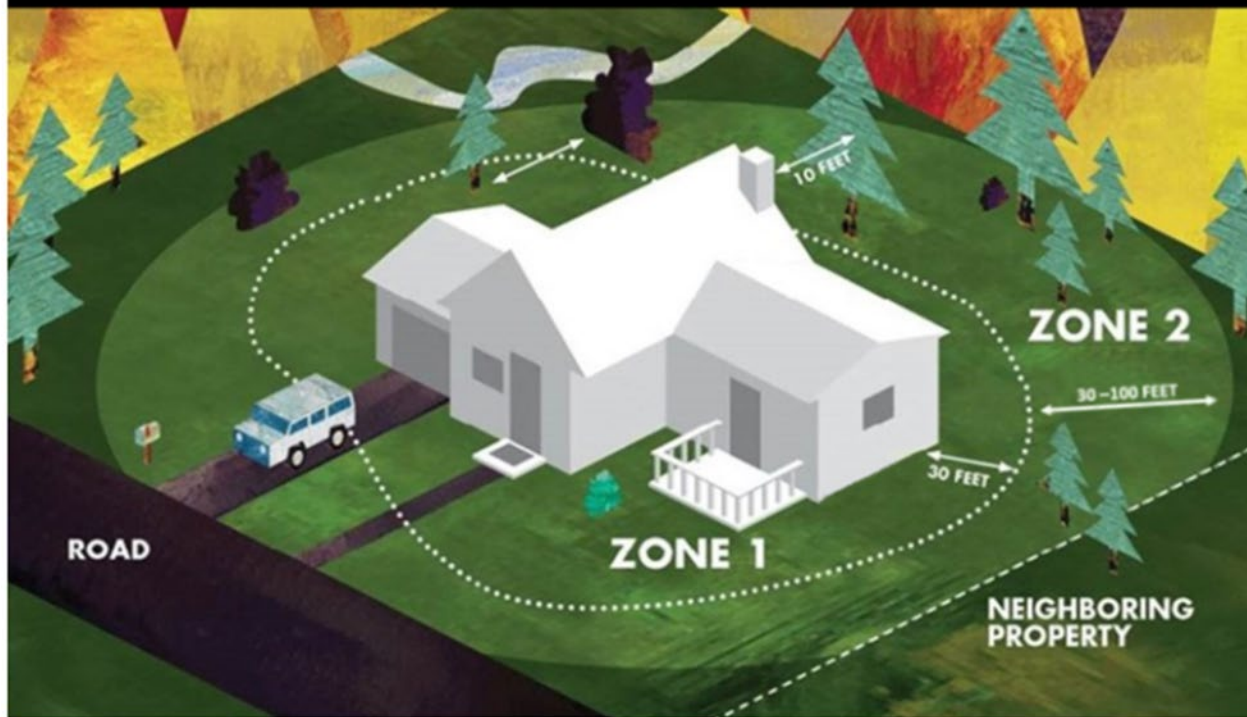
Figure 3: Idealized defensible space that is recommended around a single residential structure. This approach is often not feasible for cultural resource sites due to proximity of other structures, heritage trees, or other features that are significant to the cultural landscape.
