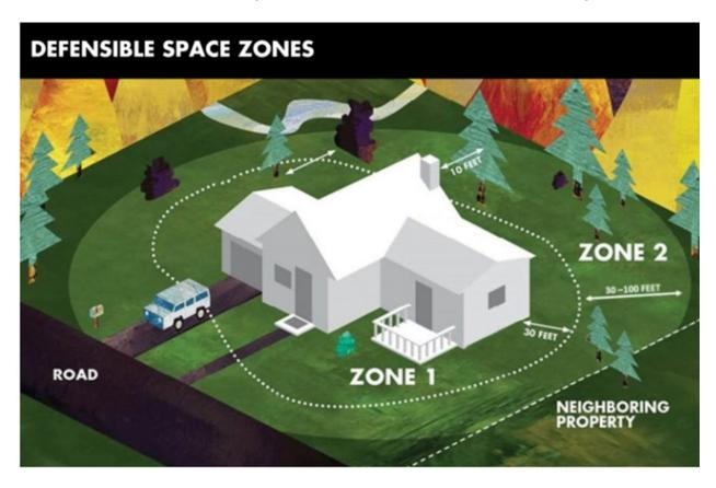
Figure 5. Idealized defensible space that is recommended around a single structure.
