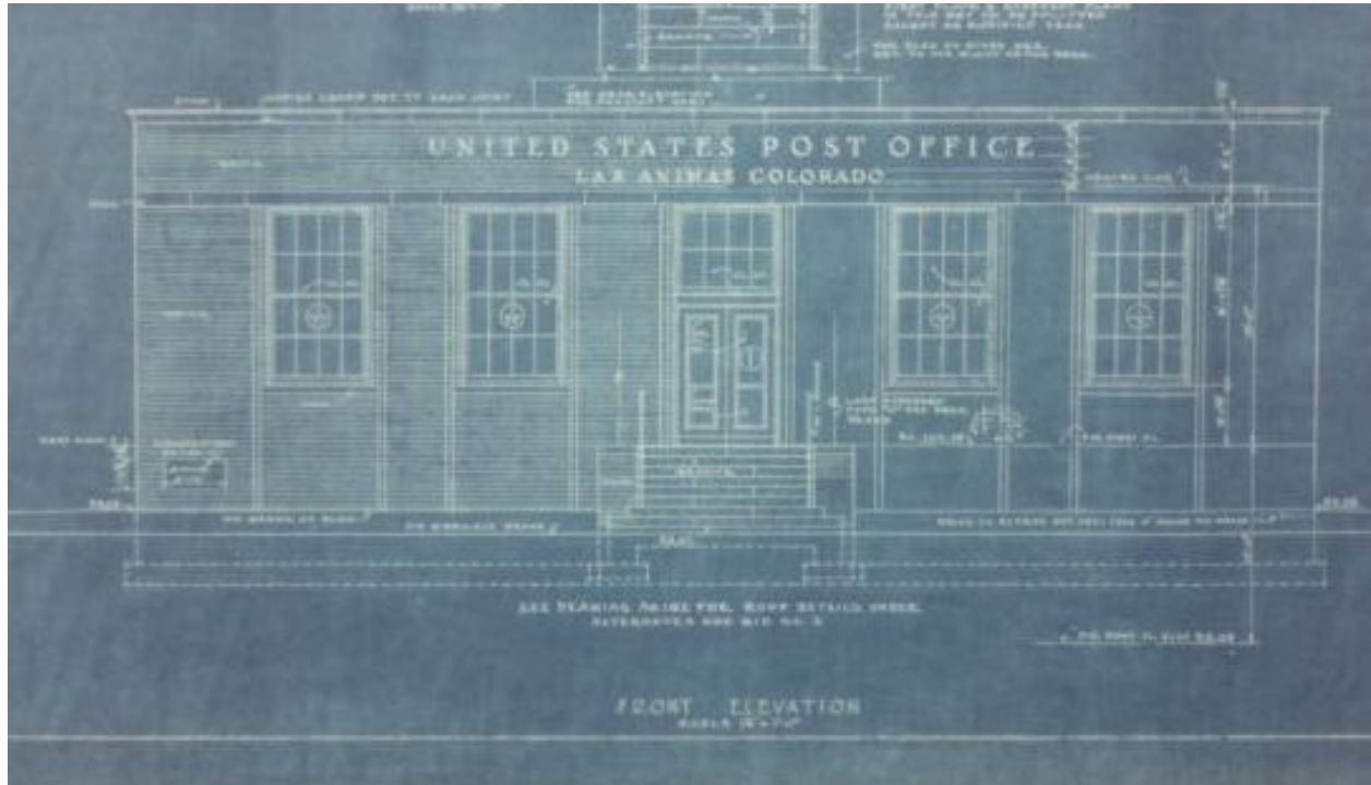
Front elevation with façade details and hipped roof
