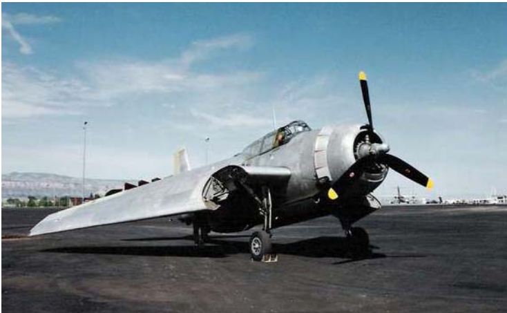
HP3. TBM N53503, aircraft exterior prior to restoration of exterior paint to World War II markings, Grand Junction, Colorado, 1989, photograph by Robert Duncan. Note wings in folded position.
