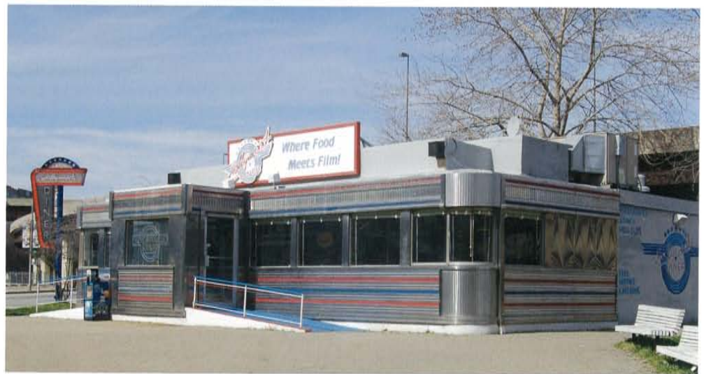
Figure 10. The shine and luster of an aluminum window with an original mill finish was a perfect complement to the stainless steel exteriors found on 1940s/1950s diners. The Hollywood Diner is an authentic Mountain View Diner built in 1954. It first operated in Westbury, New York and was later moved to Baltimore, Maryland. In the 1980s it was the location site for several Barry Levinson's films including "Diner." Most of the original windows remain in this building.
